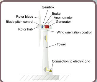
moving a magnet relative to the coil can produce a voltage as shown on the galvanometer. This voltage can then drive electrical current through standard power lines for use in homes or businesses. The illustration below shows the parts of a wind turbine.
