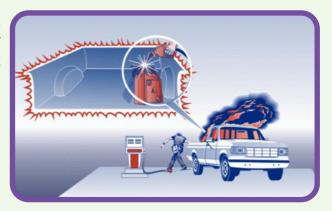
path to dissipate the static charge to the ground and reduces the possibility of fire.
